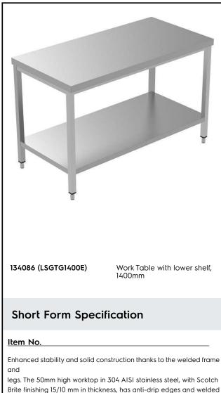
Brite finishing 15/10 mm in thickness, has anti-drip edges and welded corners. 18mm thick undertop reinforced worktop, it's completely waterproof, double-sided laminated and 100% recyclable. 40 mmthick lower welded shelf in AISI 304 stainless steel slots easily into place at a height of 200 mm from the floor (compulsory toinstall the chest of drawers). Square
